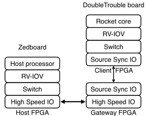
Figure 8: System level view of the two-hop system. Host FPGA (Zedboard) and Gateway/Client FPGA (DoubleTrouble)
