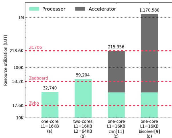
**Figure 1: Resource utilization for four Rocket cores and hardware accelerator configurations (a, b, c, and d) and available resources for supported FPGA emulation boards Zybo, Zedboard, and ZC706.**
