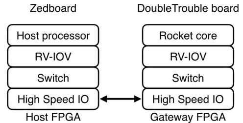
Figure 7: System level view of the one-hop system. Host FPGA (Zedboard) and Gateway FPGA (DoubleTrouble)
