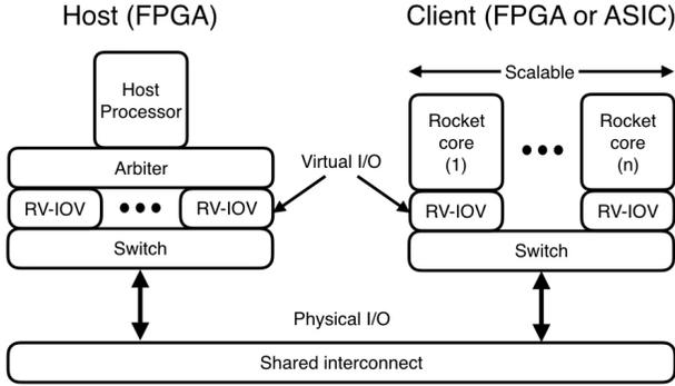
Figure 3: High level view of a RV-IOV based system.
