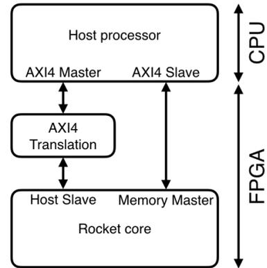
Figure 2: Rocket core emulation platform.
