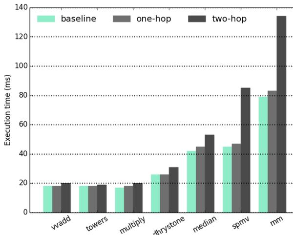
Figure 9: Execution time measured in the host for the two evaluated systems and the baseline.
