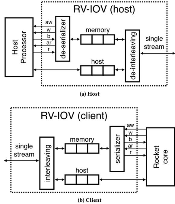
Figure 4: RV-IOV client and host architecture.
