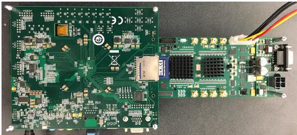
Figure 6: RV-IOV FPGA evaluation system, Zedboard (left) and DoubleTrouble (right).
