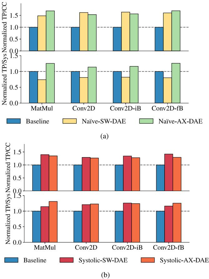
Fig. 12. Naïve and Systolic Accelerated DAE: TP/CC = throughput per compute core; TP/Sys = overall throughput per system; MatMul showing  $768 \times 768 \times 768$ ; Conv2D, Conv2D-iB, and Conv2D-fB showing 32 images batch; AddMV showing  $768 \times 768$ ; and SpMV showing FB-Johns55. See Table II for detailed input specification. (a) Naïve accelerated DAE. (b) Systolic accelerated DAE.
