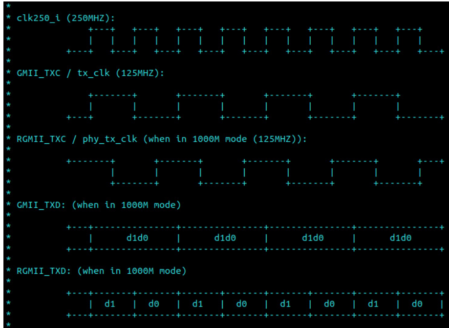
Figure 11: Waveforms for rgmii_phy_if_waveform
